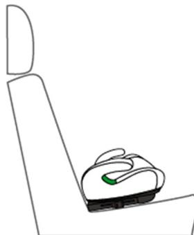
**EN** Allowed positions in car are marked in green. Always use a 3-point seat belt. Rear seat installation is recommended.
