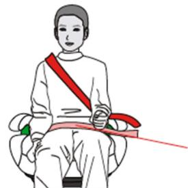
**EN** Ensure that the seat belt is threaded through the shoulder belt hook and lap belt guide at the same time.
