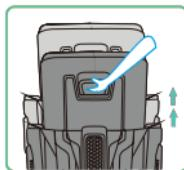
Pull up the adjustment button to adjust the height of the head rest
